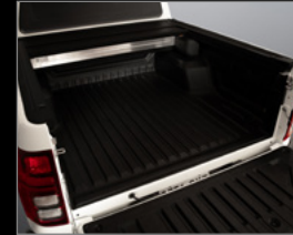
Under Rail Tub Liner
