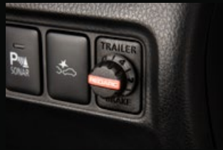
Electric Trailer Brake Controller with Harness (Redarc) #
